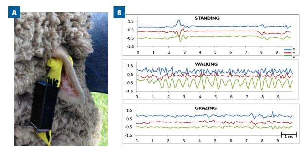
Figure 2. An accelerometer ear tag (a) and the data trace of the X,Y and Z axis demonstrating the different behaviours (b)
