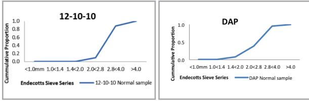
Figure 1: Cumulative sieve test Nitrophoska 12-10-10
