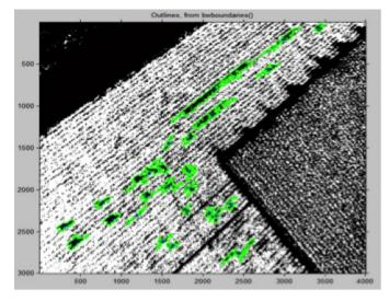
Figure 2. UAV image processing and automatic classification areas for the AgBot to direct its effort.
