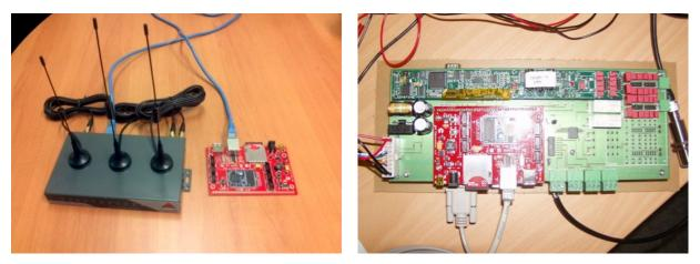
Figure 3. The 3G Wifi modem and a prototype controller board. Notable features of the board (current board shown on right) are that it incorporates all bin control, RFID multiplexing and multi-bunk/bin data sharing.
