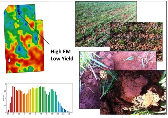
Figure 5. Ground-truthing: – High EM. The higher EM areas of the paddock are historically lower yielding. Higher EM38 sites visited had tighter more massive heavier clay profiles, lower plant establishments, reduced tillering and vigour.
