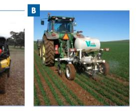
Figure 1: Veris pH detector (a) and Veris pH ManagerTM (b). The electrodes of both machines were calibrated before and after field mapping using standard buffer solutions of pH 4 and 7.
