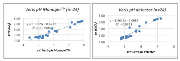
Figure 3. Correlation between the pH machine readings and laboratory pH (CaCl2).
