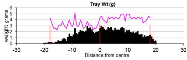
Figure 4: Spread pattern test DAP in 6ms-1 cross wind left to right
