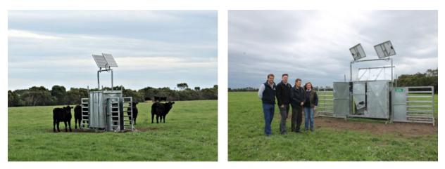
Figure 1. Twin feed bin bunker with control electronics including RFID multiplexing and multi-bunk data sharing. Trial participants (left to right): Tom Gubbins (Te Mania), Robert Wyld (Sapien), David Cottle (UNE) and Fiona Conroy (Knewleave).
