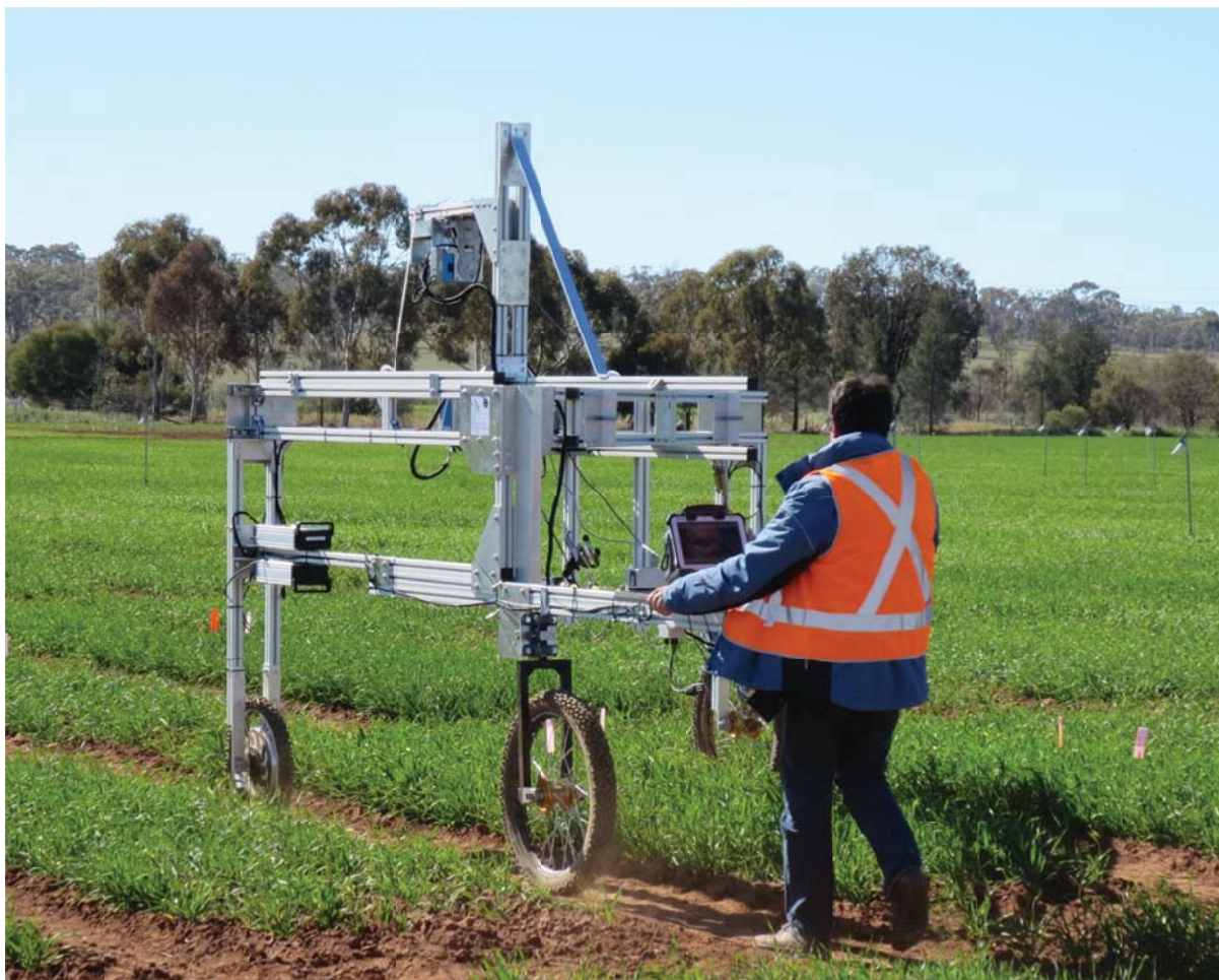
Figure 5. Phenomobile Lite scanning a breeding trial. The vehicle is hand operated and its standard operation includes a LiDAR, high-resolution camera and Greenseeker ® NDVI sensor.
