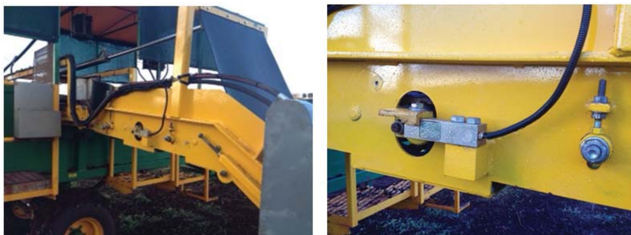
Figure 2. Load cell position on harvest platform.
