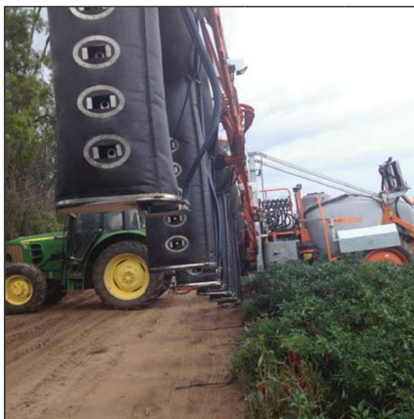
Figure 4. Greenseeker sensors mounted to a custom spray boom for chillies.
