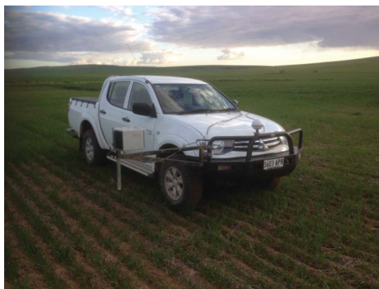
Figure 1. The H-Sensor mounted to the ute for mapping and collecting images of the crop and weeds.
