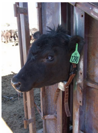
Figure 1. Photograph of the UNTracker collar. Note the receiving antenna is located out of view on the top of the collar. The polycarbonate box housing the hardware and battery acts as a counterweight to maintain the GPS receiver antenna on top of the animal's neck.
