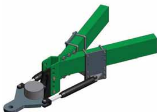
Figure 3. The iTill hydraulic implement steering design (a) and an early season image of a production trial (b).
